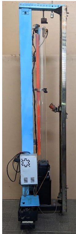
Figure 11. The web-remote laboratory-based free fall motion experiment automation device after the improvements.
