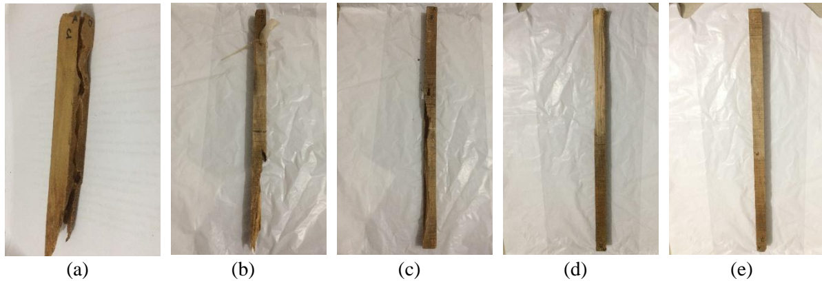
Figure 3. Damage value of wood sample due to M. gilvus termite attacks (a) 0, (b) 4, (c) 7, (d) 9, and (e) 10
