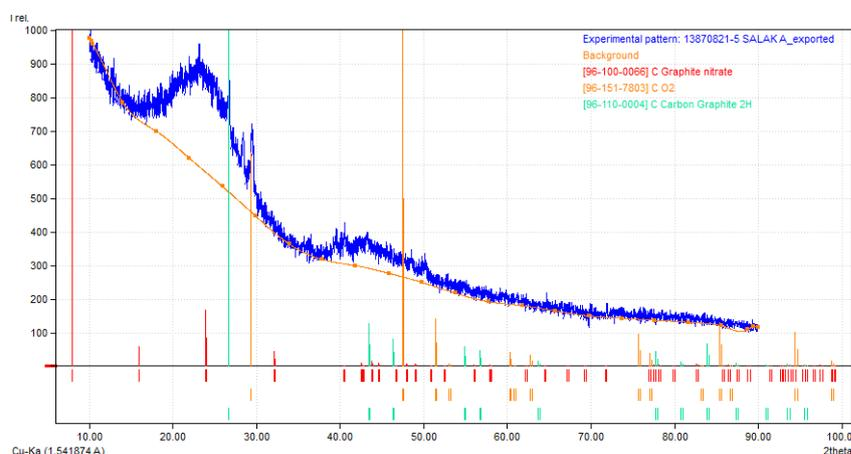
Figure 4. Identification results using the Match! software
