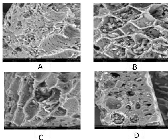
Figure 1. SEM results. (a) bark carbon with  $KOH$  activation (b) bark carbon with  $ZnCl_2$  activation (c) bark carbon with graded activator Carbon  $ZnCl_2 + KOH$  (s) (d) bark carbon with graded activator Carbon  $KOH + ZnCl_2$  (s)
